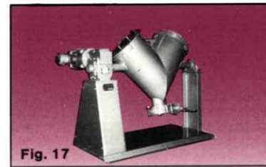
Fig. 17 1 CU. FT. LABORATORY VEE BLENDER.
